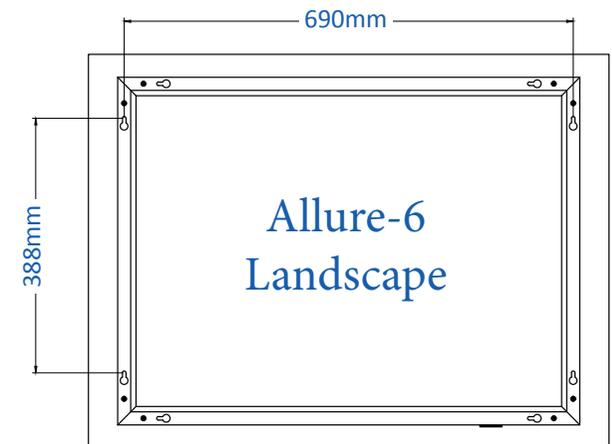
The drawings above shows the dimensions for wall drillings for the installation of the mirror
